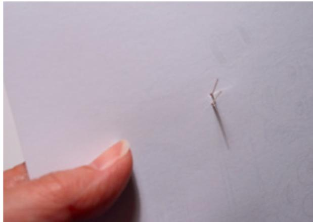
5. Pull the LED all the way through the card so the bottom of the LED is flush with the card.
